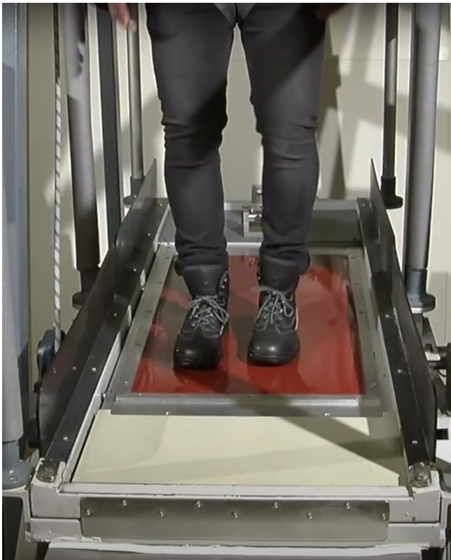
Fig. 3: R-value ramp test taken from Altro slip-resistance test guide video
