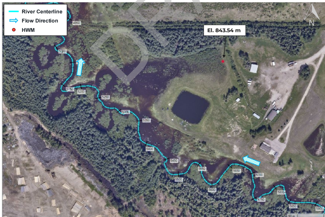
Figure 4-2 (d): HWMs Identified from Mudlines in 2023 Flood Aerial Imagery Located North of the Dugout
