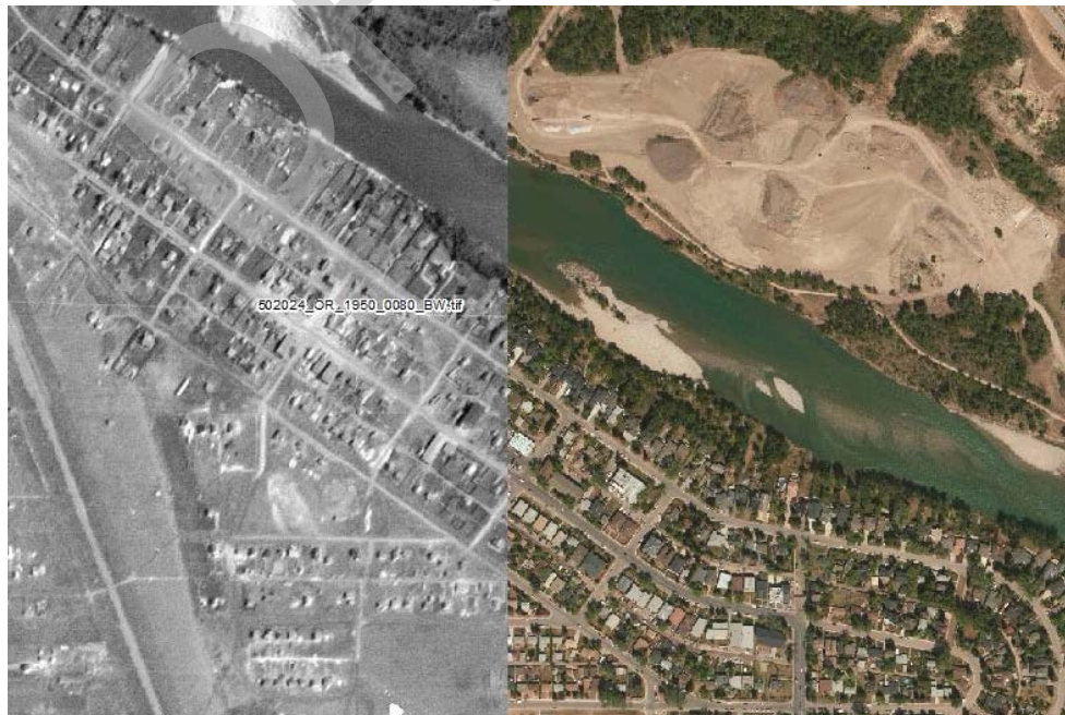
Figure 1: Example of an Orthomosaic Quality Assurance Check at 1:5,000 Scale (The historical 1950 orthomosaic (greyscale image; at left) is peeled back to reveal the modern landscape (colour image; at right)
