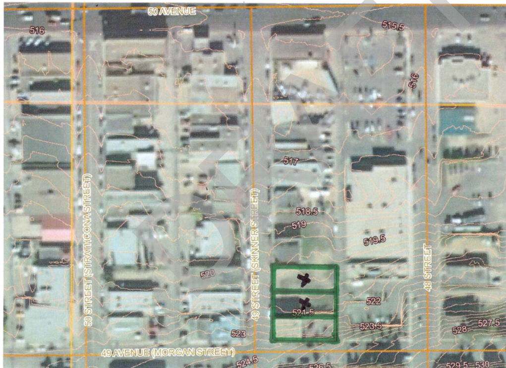
Figure I-19. Present day lot locations of the relocated HBC warehouses, east of 49 th (Skinner) Street. The green lines represent approximate lot lines and the Xs mark the intended locations of the structures. The minimum elevation of the most northerly lot was about 520.0 m.
