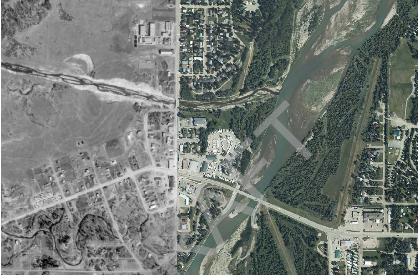
Figure 1: Example of an Orthomosaic Quality Assurance Check at 1:5,000 scale. The historical 1962/1963 orthomosaic (greyscale on left) is peeled back to reveal the modern landscape (colour image on right).
