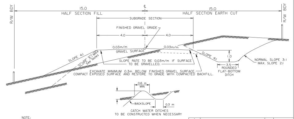
SERVICE ROADS ARE GENERALLY GRAVEL SURFACED AND 8m WIDE AS SHOWN HERE UNLESS CARRYING HIGH TRAFFIC VOLUMES. HIGHER VOLUMES MAY DICTATE THE NEED FOR A PAVED SURFACE AND/OR A WIDER ROADWAY AS PER NORMAL DESIGN PRACTICE. LOWER DESIGN SPEED MAY BE USED WHERE APPROPRIATE AS PER GUIDELINES IN CHAPTER H (LOCAL ROADS) OF THE HIGHWAY GEOMETRIC DESIGN GUIDE.
