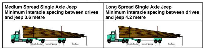
7 Axle Tandem Jeep / B-Train: a configuration having two trailers - one trailer can be a tandem jeep with a tandem trailer, or it may be a configuration with a single trailer with two separate tandem axle groups.
