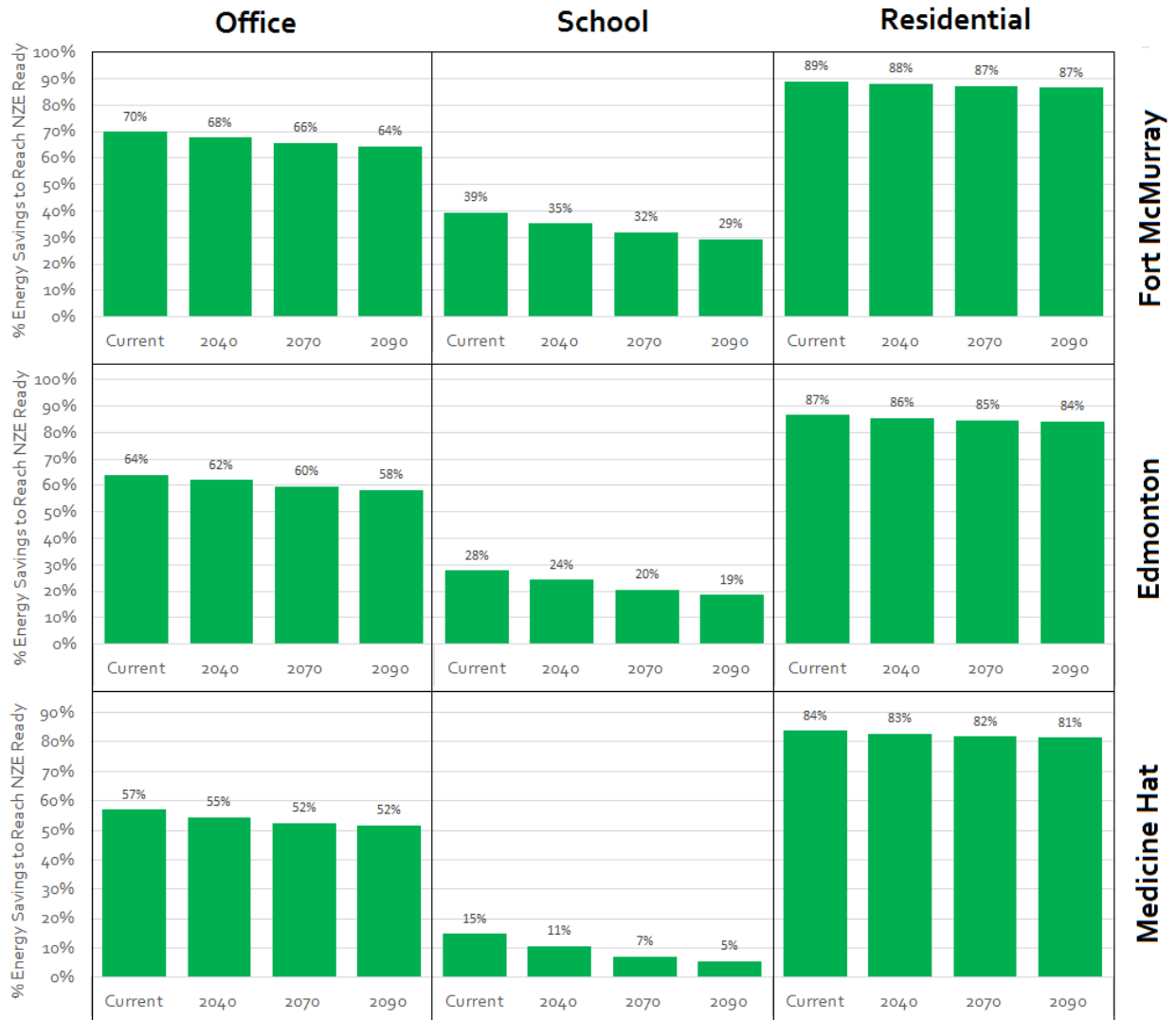
Figure 18 Percentage energy savings from baseline required to reach net-zero ready for RCP8.5
