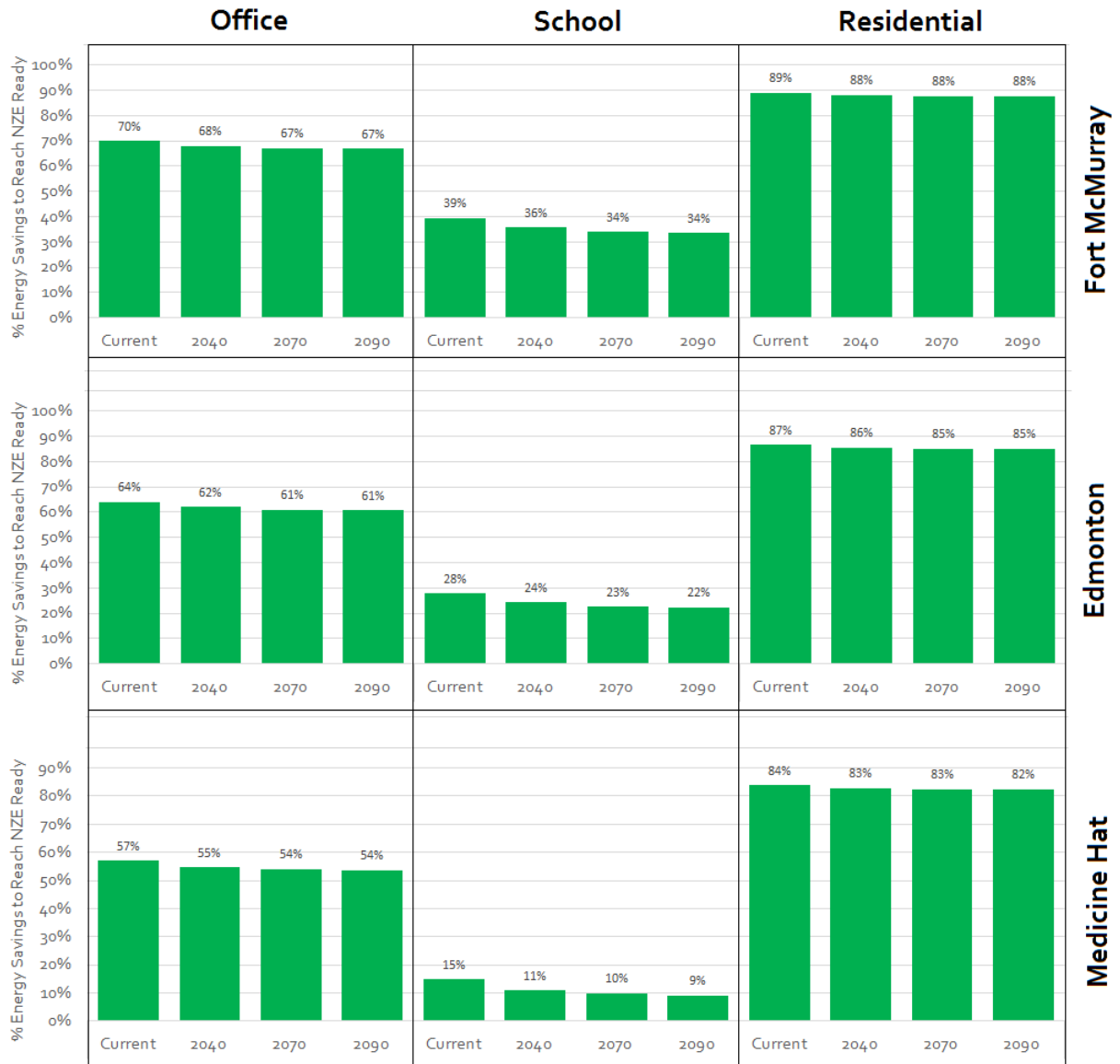
Figure 19 Percentage energy savings from baseline required to reach net-zero ready for RCP4.5
