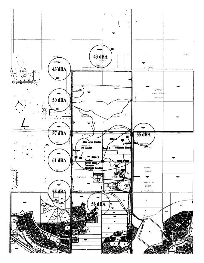
Figure 1: Noise Projections With An East Wind For Continuous Operations At The Spy Hill Development Located On Section 28 (Scraper Noise Not Included)
