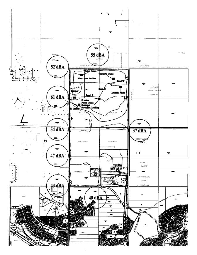
Figure 2: Noise Projections With An East Wind For Continuous Operations At The Spy Hill Development Located On Section 33(Scrapers Not Included)
