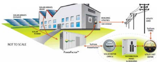
Figure 4 - Islandable microgrid – Photo credit – Solar Grid
