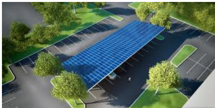
Figure 13 – Covered parking with Solar PV array
