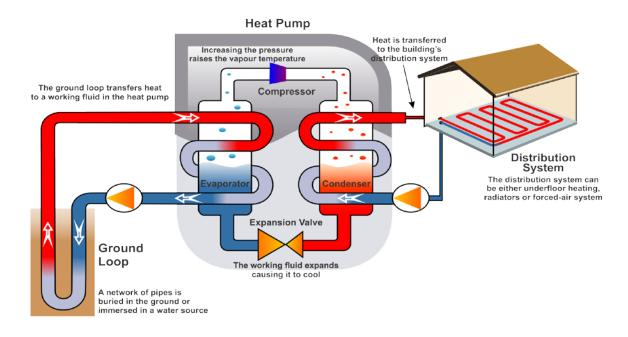
Figure 14 – Schematic of a Geothermal Heat Pump - Photo credit – Google.
