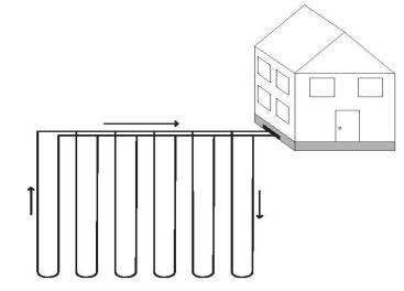
Figure 8 – Vertical closed loop heat exchanger for a geothermal heat pump - Photo credit – Self et al., 2013.
