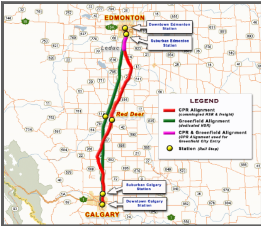
Exhibit 1.1: Calgary-Edmonton High-Speed Rail Alignment Alternatives
