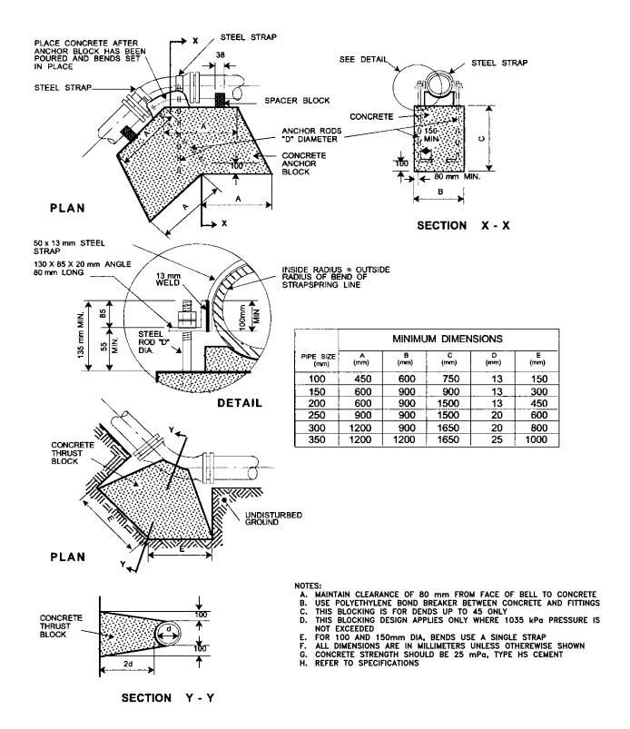
Vertical Thrust Block Detail
