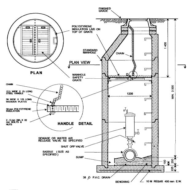
NOTES: WHEN USING PVC PIPE, INSTALL PVC MANHOLE ADAPTER. WATERPROOF EXTERIOR SURFACE OF MANHOLE WITH MATERIAL SPECIFIED
