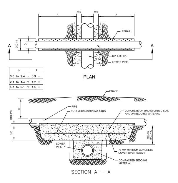
NOTE: PLACE POLYETHYLENE SHEET BETWEEN LOWER PIPE & CONCRETE. IF CROSSING A 3RD PARTY UTILITY, CONFIRM REQUIREMENTS AS PER CROSSING AGREEMENT
