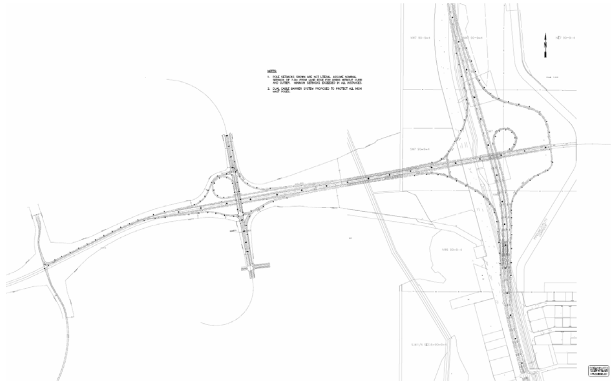
Preliminary Lighting Layout, 35 m High Mast Poles
