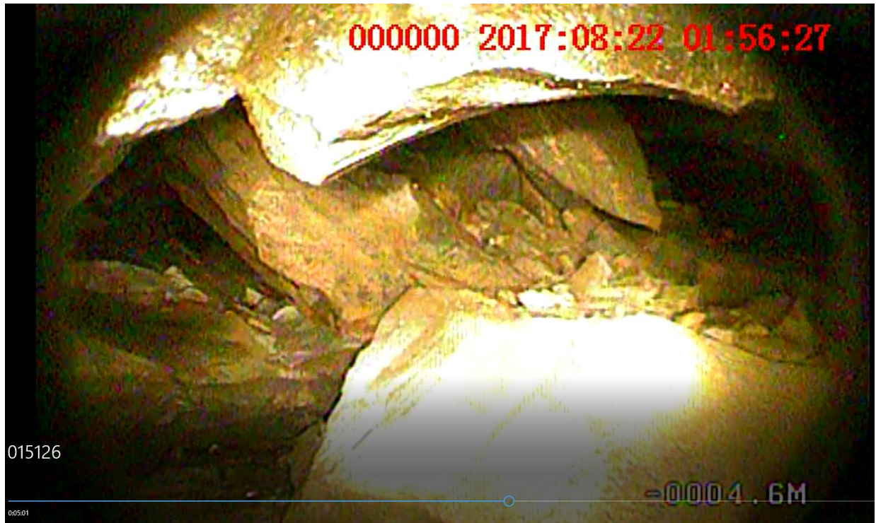
Figure 7. Image from 2017 downhole-video-camera survey of metal-capped borehole. Note roof collapse material.
