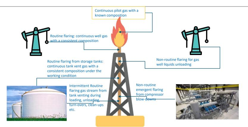
Figure: An Example of Multiple Flaring Streams
