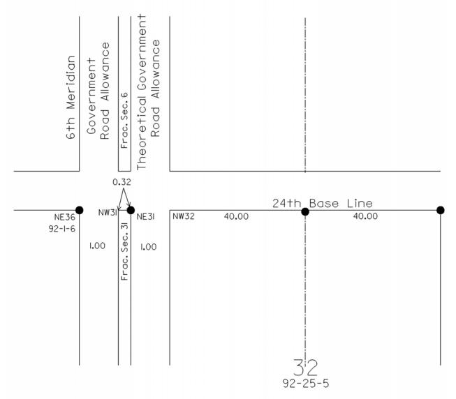
Note: This layout is as shown on the current Base Line plan confirmed June 2,1954. The Base Line appears to have been drafted in error. It does not agree with the field notes and the actual position of the NE31 as tied on several subsequent plans (see appendix "A"). Diagram not to scale.
