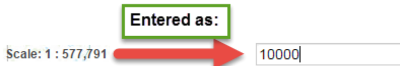
Figure 4. Illustrates how to produce a 1:10,000 scale map from the soil viewer map area at displayed at a scale of 1:577,791
