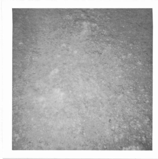
**Figure 6: Pitted or Pock-marked Appearance Due to Coarse Aggregate Loss**
