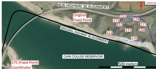
Figure 8. GPS Unit Location on Chin Coulee (base imagery from ESRI, 2019)
