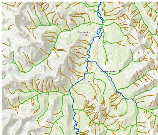
Figure 4. Statistically predicted debris flow (brown), debris flood (green) and flood (blue) stream process types near Kananaskis Village.
