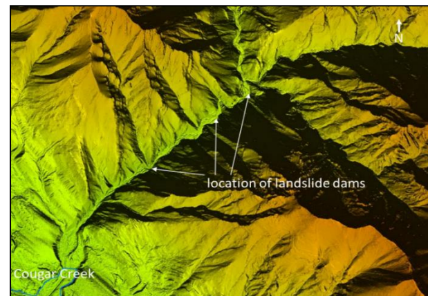
Figure 10. Example of evidence for landslide dam outbreak flood potential in Cougar Creek basin.
