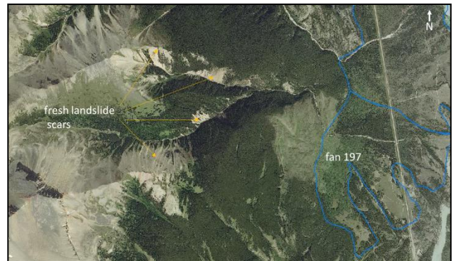
Figure 6. Example of evidence for recent landslide activity within the basin of Fan No. 197.
