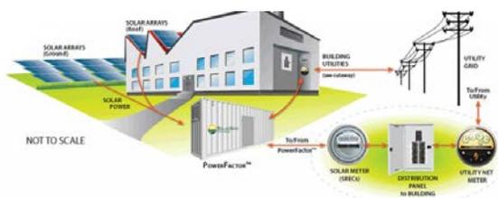
Figure 4 - Islandable microgrid – Photo credit – Solar Grid
