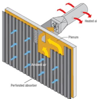
Figure 10 – Solar wall schematic – Photo credit – Google
