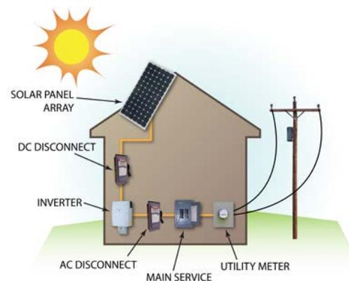
Figure 3 – PV Modules Net Metered Arrangement -
