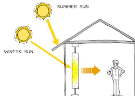
Figure 11 – Trombe wall schematic – Photo credit - Google
