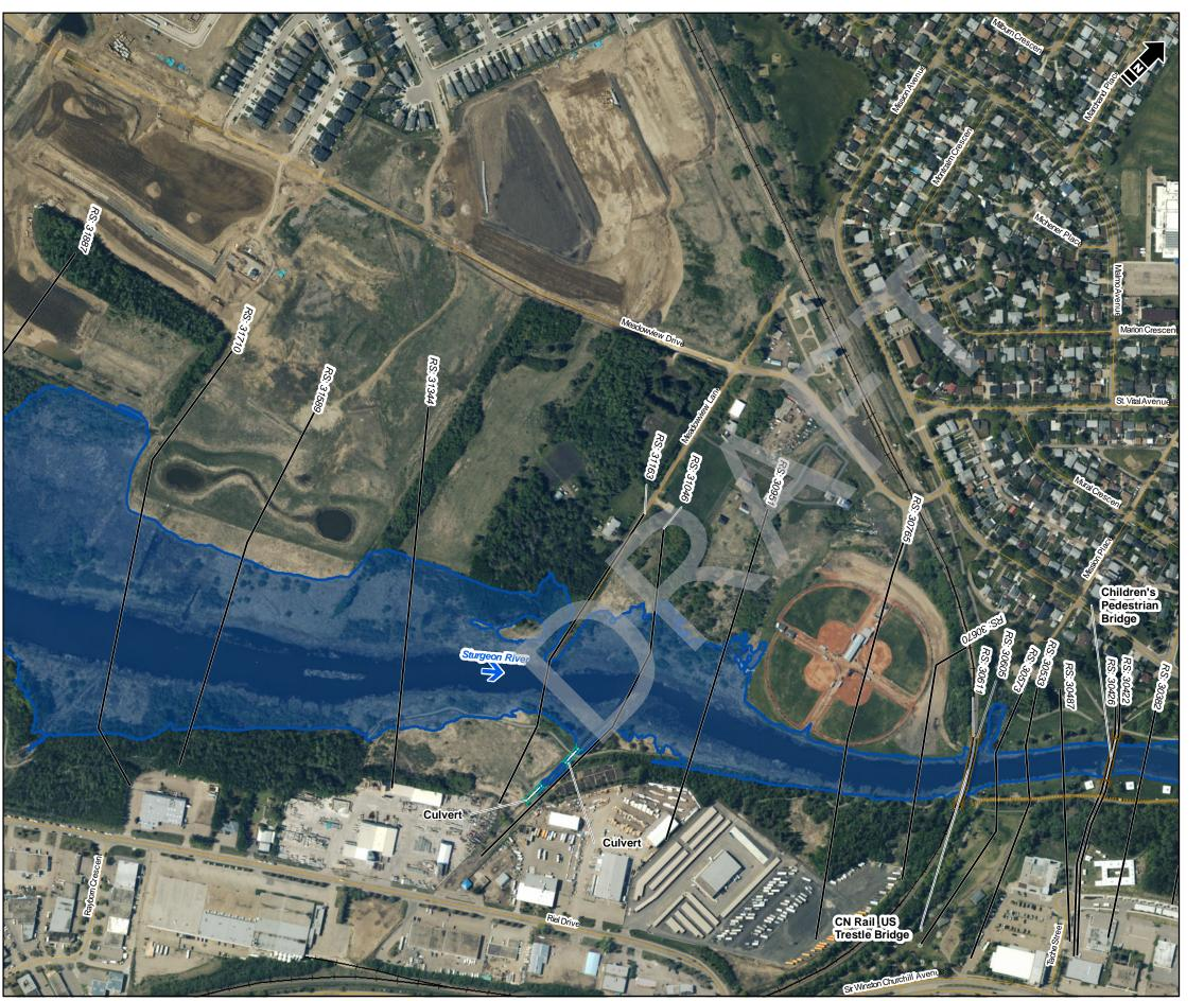
Bridge Culvert --- Cross Section Line -- Study Mapping Limit Flood Control Structure ---- Municipal Boundary (Urban) ---- Municipal Boundary (Rural) --- Major Road — Local Road — Railway Flow Direction 5-Year Flood Inundation Extent 5-Year Flood Inundation Extent (Potential Flood Control Structure Failure)
