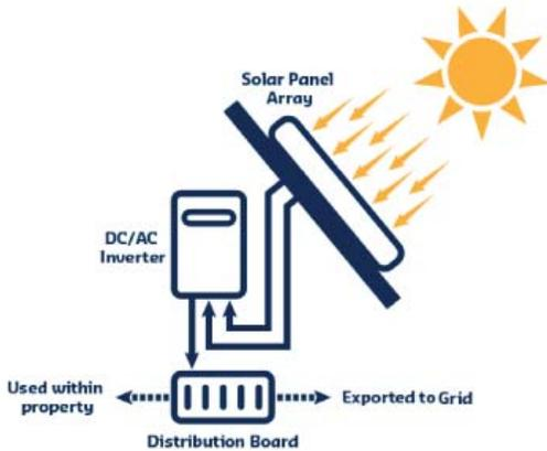
Schematic of Photovoltaic System (Roof or BIPV)
